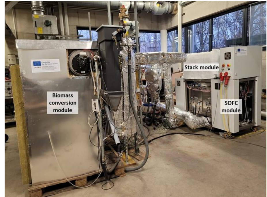
Micro-Bio-CHP plant at site of project coordinator BIOS in Graz
